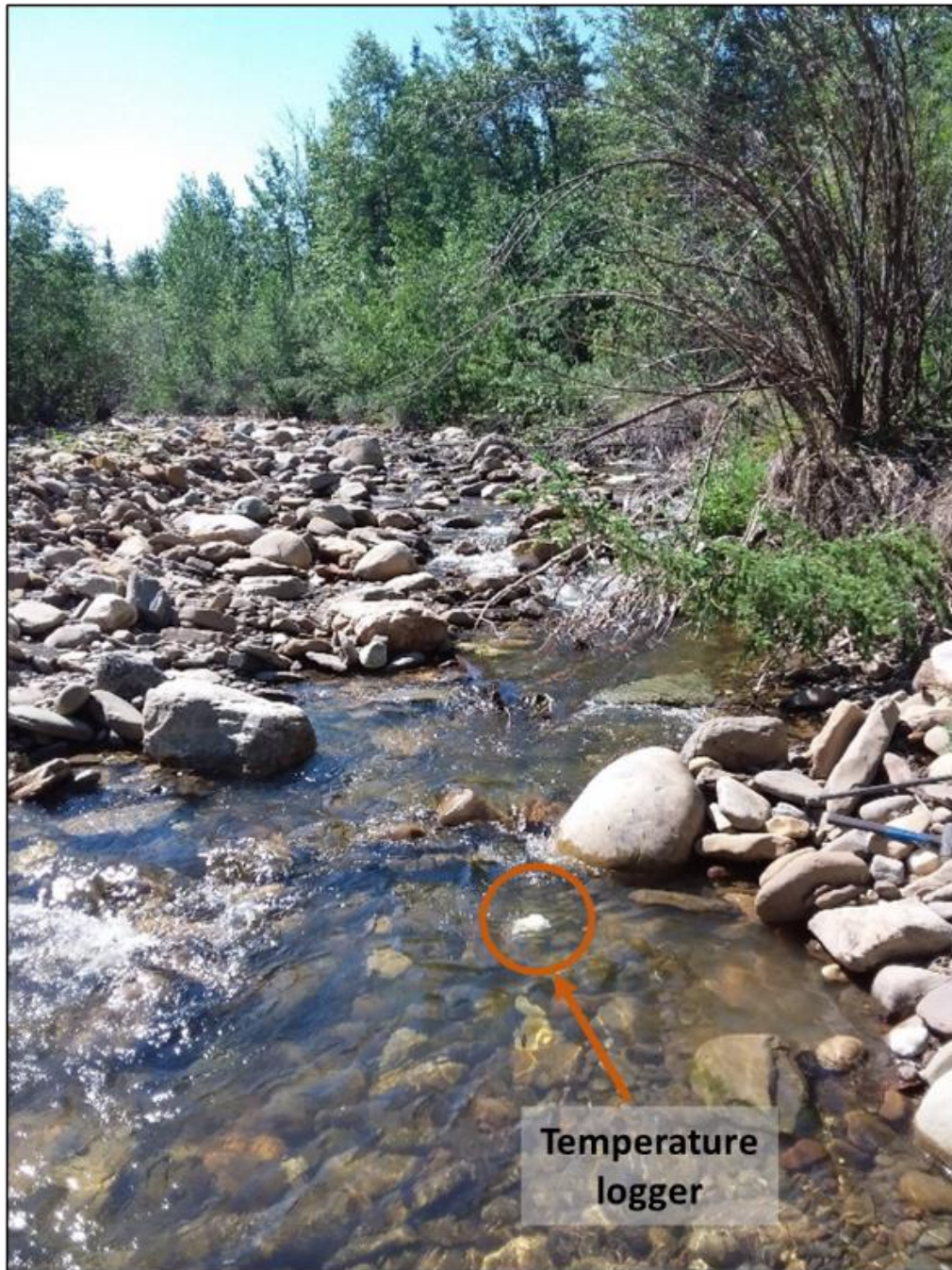
Figure A1. Example of a temperature logger installation at a monitoring site (STC1). Location of the logger is outside the main thalweg, behind a large sturdy boulder to protect it from debris flows, within the perennial confined channel and at a depth where can be easily retrieved if water levels rise.
